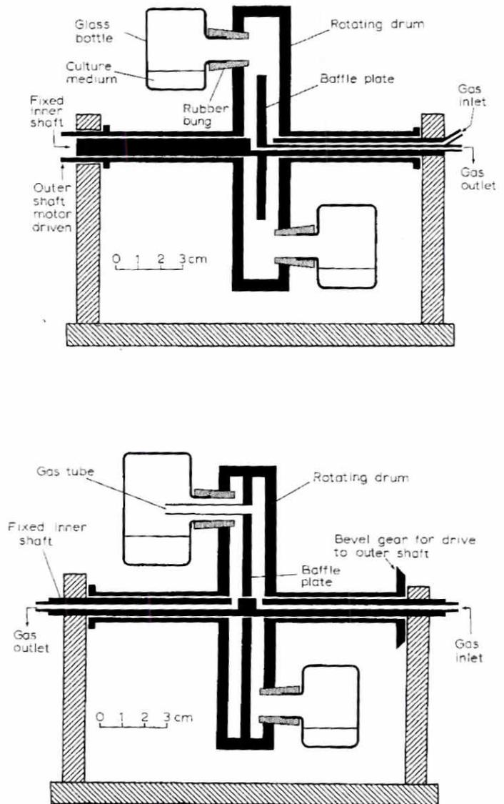
**Fig. 6. Cross sections of two types of rotator apparatus.** Two models of rotator apparatus, in which the rotating bottles are constantly gassed by diffusion (upper diagram) or via tubes projecting into the bottles (lower diagram). (From New and Cockroft, 1979).
