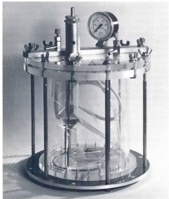
**Fig. 4. Pressure chamber apparatus.** Pressure chamber containing circulators that can operate at two or three atmospheres of pressure.
