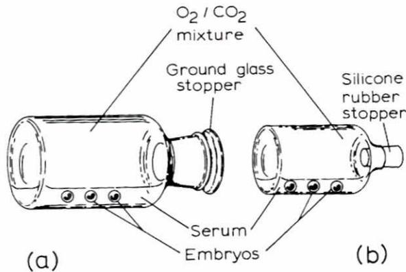
**Fig. 5. Two types of roller bottle cultures:** The bottle shown in (a) is a standard 60 ml reagent bottle sealed with a little silicone grease around the glass stopper, whilst that in (b) is a purpose made Pyrex bottle, sealed with a silicone rubber bung. (From Cockroft, 1990).
