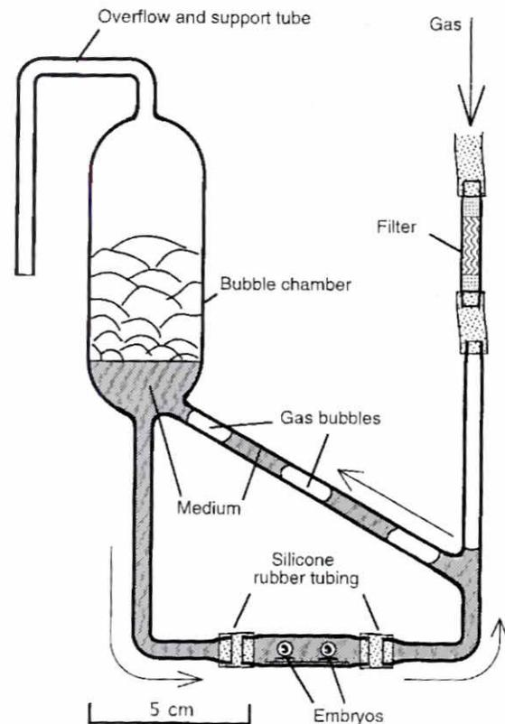
**Fig. 2. Circulator culture apparatus.** A device for growing embryos in oxygenated flowing medium. Arrows indicate the direction of gas and medium flow.
