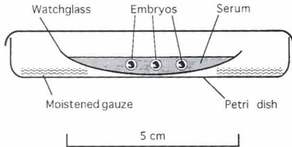
**Fig. 1. Watchglass culture apparatus:** several of these can be stacked in a gas-tight chamber within the incubator.
