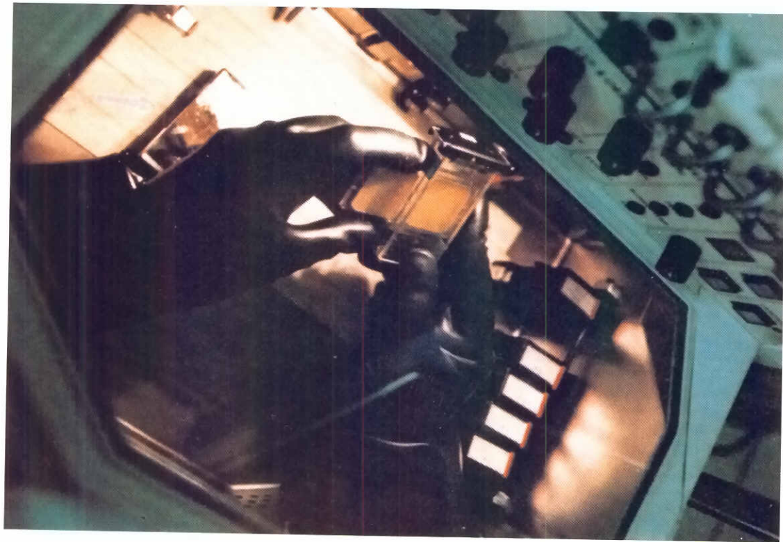
Fig. 2. Hardware of the biorack Fly 15 Experiment: Type I experimental and tray holding containers. The trays were labeled with different colors to be matched with the colors in the containers to minimize possible mistakes in the operating protocol. Below, the Biorack with the operation of the tray exchange. These photographs were kindly supplied to the authors by the European Space Agency.
