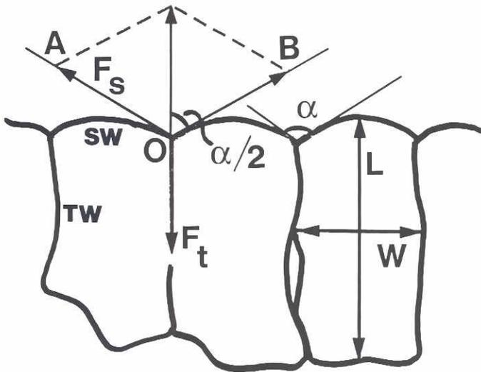
**Fig. 12.** Drawing of measurements taken of cell surface angles ( $\alpha = \text{AOB}$ ) and of columnarization indexes ( $\text{IC} = L/W$ ).  $OA$  and  $OB$  are the tangents to cell surfaces at apex point  $O$ . Forces of cell surface tension  $F_s$  oriented along the tangents to the cell surface are assumed to be equilibrated by force  $F_t$  of transversal cell wall tension.  $sw$  - surface wall,  $tw$  - transversal wall.
