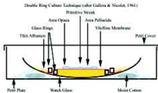
Fig. 4. The double-ring culture technique (after Gallera and Nicolet, 1961).
